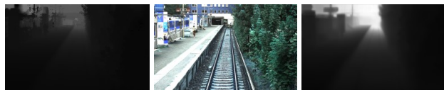
Fig. 4: Depth estimation module prediction example (absolute depth). Left: Ground truth, Center: Input, and Right: Prediction.
