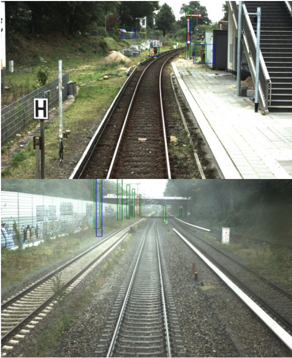
Fig. 6: Examples of detections made by MFF, green boxes represent GTs, blue boxes represent short-range 3D object predictions and red boxes represent long-range 3D object predictions.
