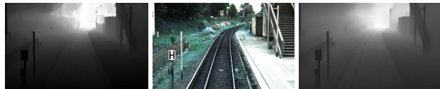
Fig. 3: Depth estimation module prediction example (relative depth). Left: Ground truth, Center: Input, and Right: Prediction.
